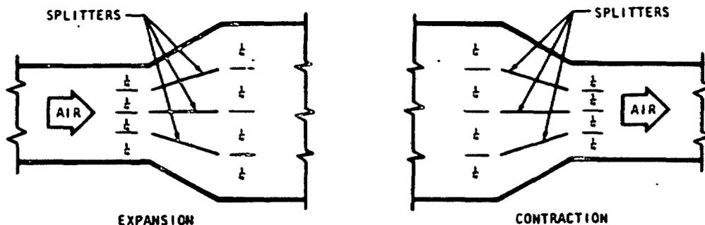
FIGURE 4-3. Splitters in expansion and contracting fittings.
