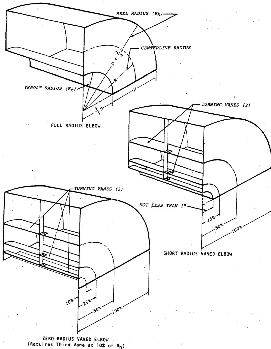
FIGURE 4-4. Curved elbows for rectangular ducting.
