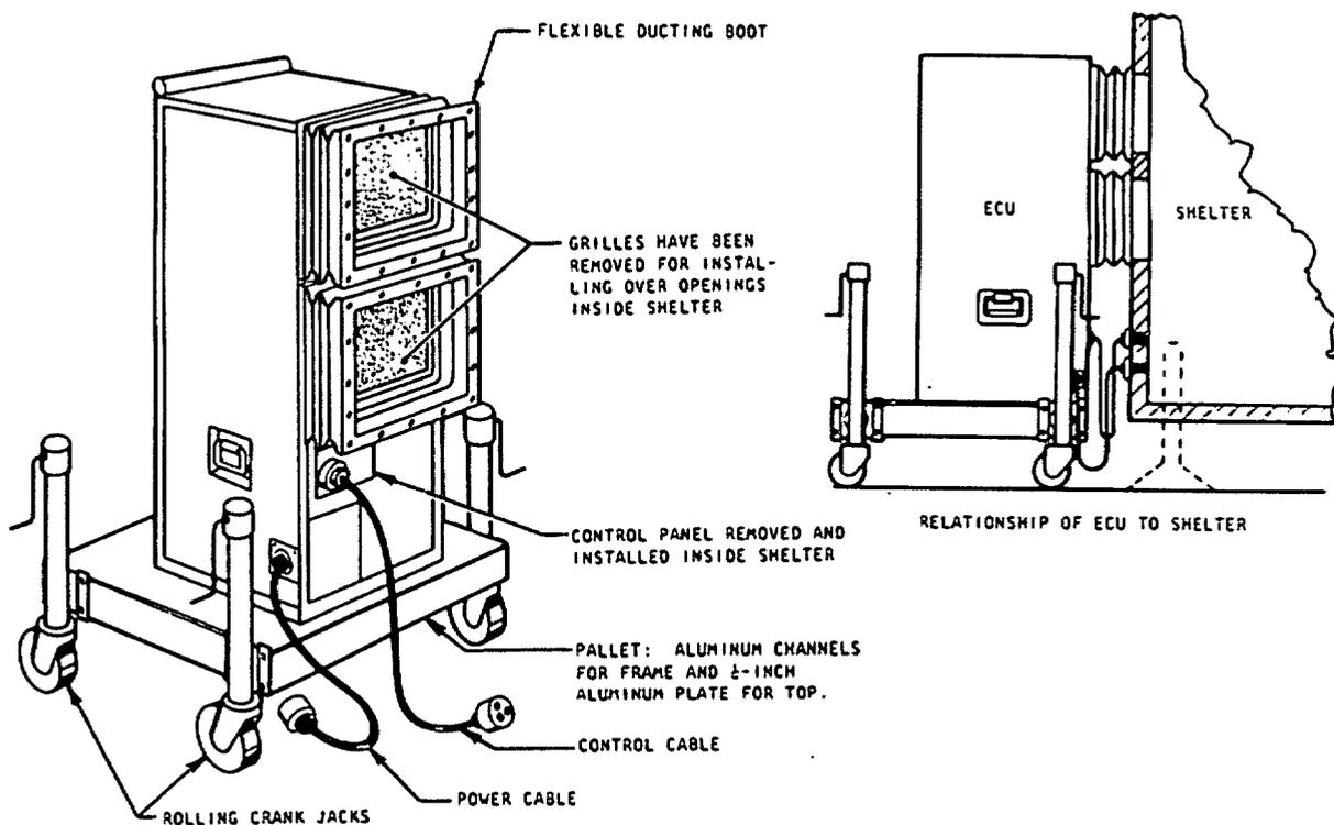
Major actions to place into operation: Remove grilles from ECU; attach boot to ECU; attach power cables; push ECU into position close to shelter; attach necessary gasketing; attach boot to shelter; attach necessary filters; attach grilles to opening inside shelter; attach necessary tiedowns.
