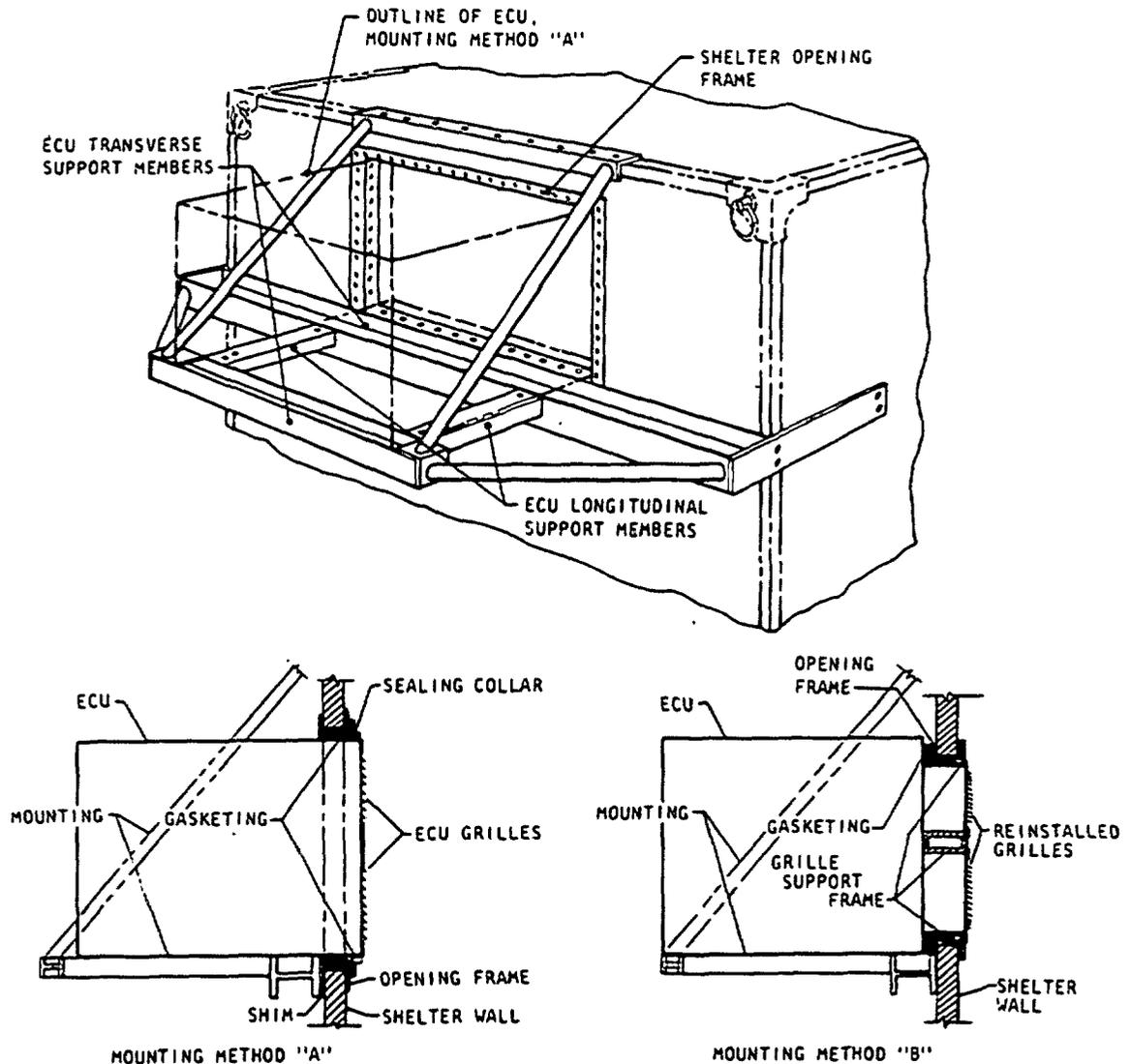
ECU fits through opening into shelter. This is simpler of two methods but it is a little more difficult to seal.
