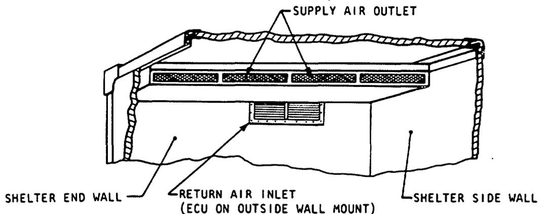
FIGURE 4-7. Outlet for reducing air velocity and noise.
