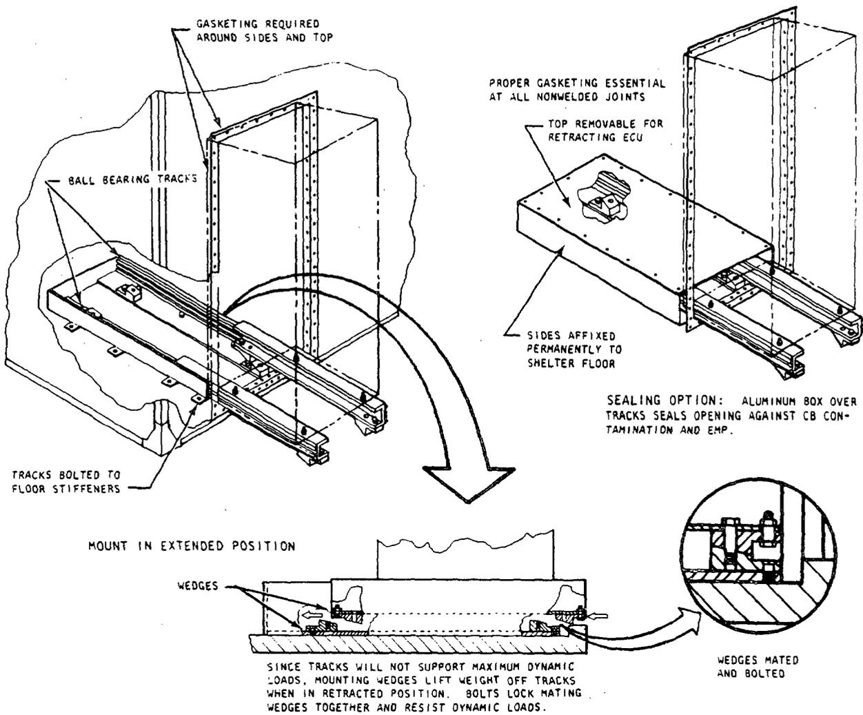
Major actions to place into operation: Remove plug from wall opening; push ECU into operating position; attach bracing as required; place cover plate over tracks inside shelter (for sealing); attach power and control cables; attach any ducting required; start ECU.
