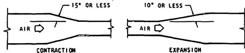
FIGURE 4-2. Maximum desirable contraction and expansion angles.
