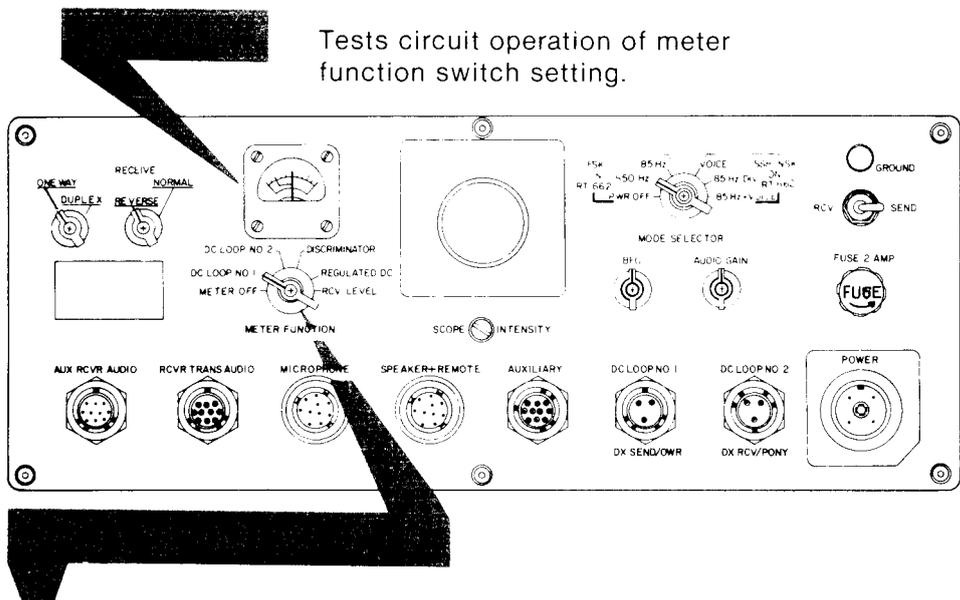
Tests circuit operation of meter function switch setting.
