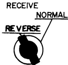
Check teletypewriter machine printout. If you cannot read the printout, place modem RECEIVE switch at REVERSE.
