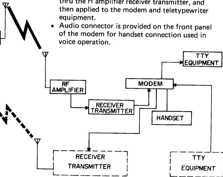
In DUPLEX operation, an additional teletypewriter and receiver-transmitter is required. This enables the system to transmit and receive at the same time.
