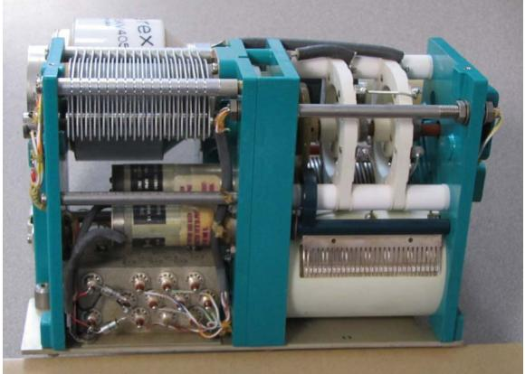
Have arcing and smoking from the turret? If so, the 2A2 turret blades and the matching 2A9 stator contacts are most likely burnt or
