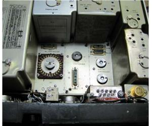
If not, get a .050 Allen wrench and adjust them. If OK, turn over the modules and make sure each module's pin or slot is also pointing to its "0" index mark
