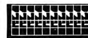
l. 1.50-KHZ KEYING PULSE IA6A2E5 1 VOLT/CM 20 MICROSECONDS/CM
