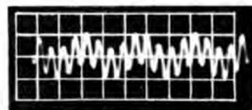
g. 1.97-MHZ PLUS 9.07 MC OUTPUT IA4A2E9 0.05 VOLTS/CM 0.2 MICROSECONDS/CM (1.981MHZ FOR RT-834/GRC)
